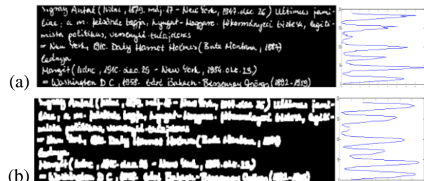
Figure 8 Horizontal Histogram Projection of the Images: (a) projection of the original image, (b) projection of the smoothed image
