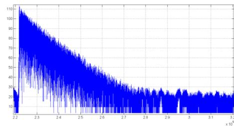
Figure 10. Signal pistol shot decay waveform (microphone in the centre of camera), RT60 is about 0.56sec, frequency of samples is 65536Hz
