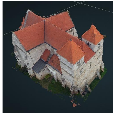
Figure 5. Potree viewer with the point cloud about the ancient cathedral in Ócsa
