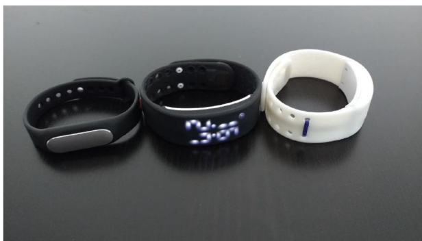
Fig. 1. The devices used during the measures. From left to right, Xiaomi Mi Band, and W2 devices. The W2 devices were labeled with a special string, and that was used as color code of a given device.
