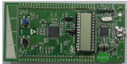
Figure 11. The circuit board module matching based on the microcontroller STM32L-Discovery
