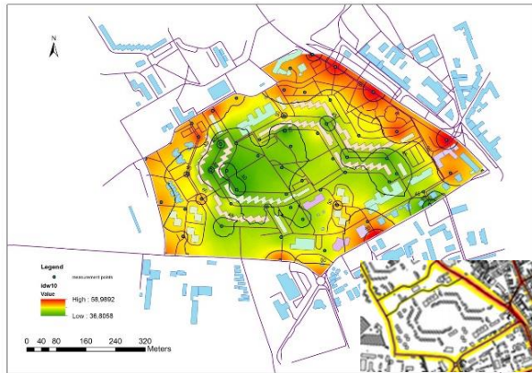
Figure 5: The results of the noise measurements with the official noise map [7] in the bottom right corner.
