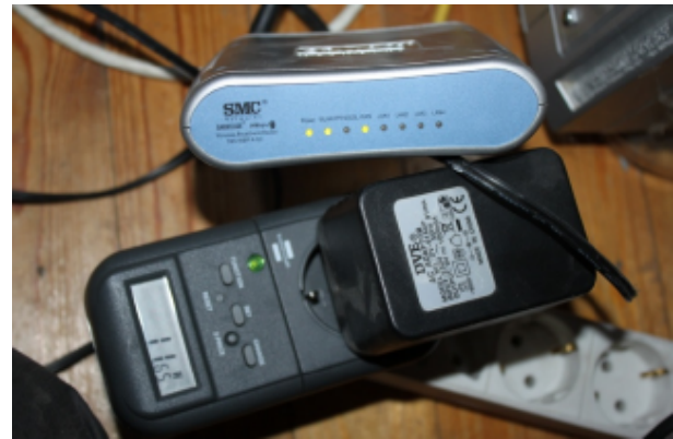
Fig. 2. Electric consumption analyzing of home wireless router in standby mode.
