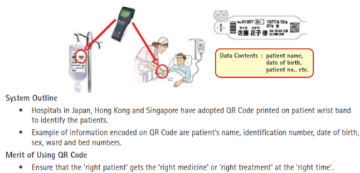
Figure 8. QR Code Used For Patient Identification in Japan, Hong Kong and Singapore
