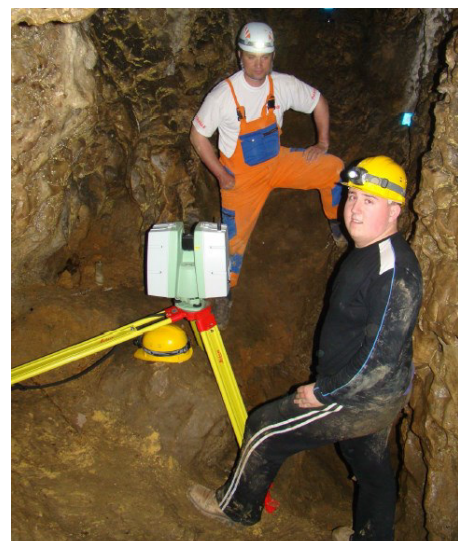
Figure 2. A laser scanner in the Cseszneki-cave
