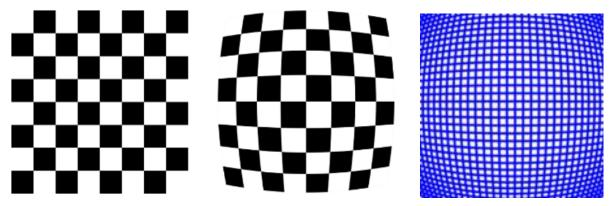
Figure 10: positive radial distortion (a: calibration pattern, b:barrel distortion, c: model)
