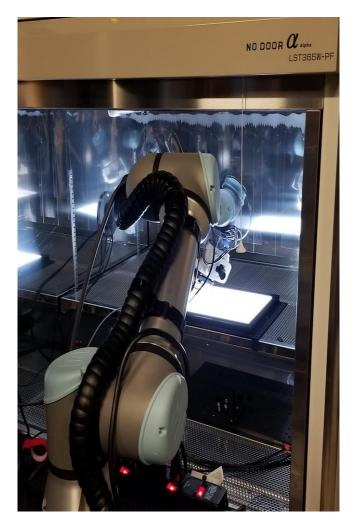
Figure 23 Sensor assembly positioned by articulated robot arm in temperature chamber
