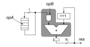
Figure 79. Bit-serial multiplier
