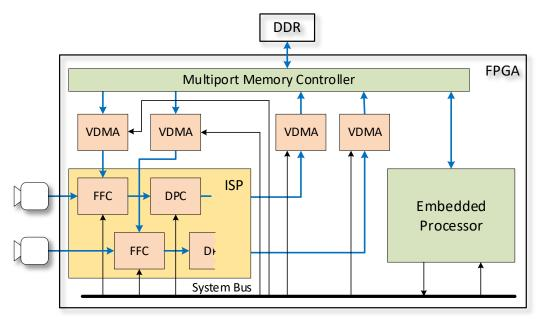
Figure 26. Uniformity correction solution for stereo cameras
