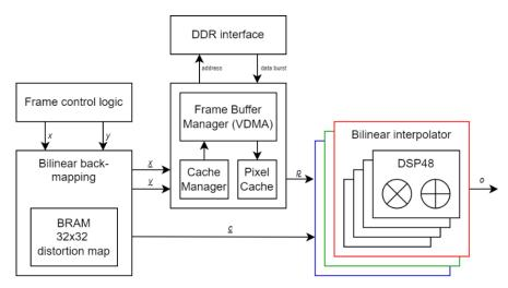
Figure 13: Block diagram of a lens-distortion correction module for Xilinx FPGAs
