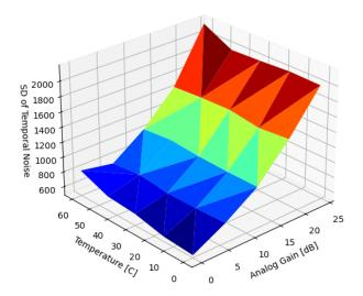
Figure 35. Standard deviation of temporal noise  $\sigma_t(\alpha, T)$
