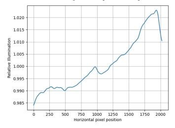
Figure 41. HIP of LSC without de-center correction
