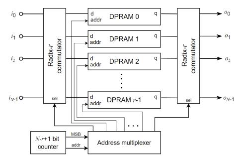
Figure 72: Example of a r input, r-output, data reorganizer for radix-r FFTs
