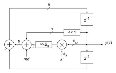
Figure 98. Constrained Multiplier
