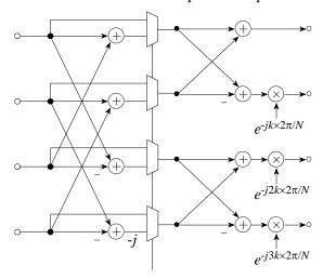
Figure 93. Radix-4 PE with bypass-option
