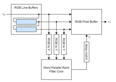
Figure 63: Word parallel rank-filter architecture for RGB color image processing
