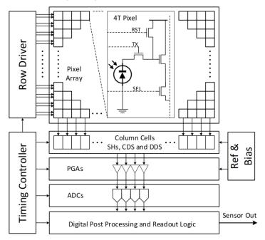
Figure 19. Typical CMOS image sensor block diagram
