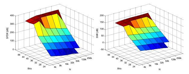
Figure 78. SFDR (left) and SNR (right) as a function of N and B, M=128
