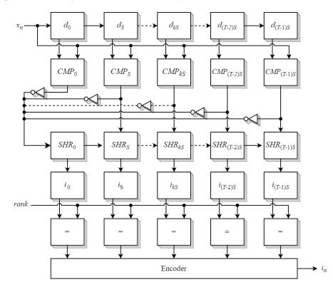
Figure 64: Word-parallel filter core architecture
