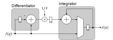
Figure 76. DI structure with preload
