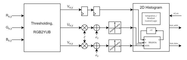
Figure 54: Illuminator estimation specific hardware components in the Image Statistics ISP Module
