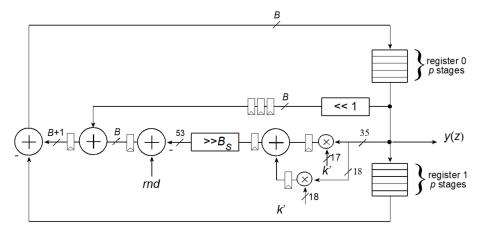
Figure 99. Pipelined resonator using block multipliers
