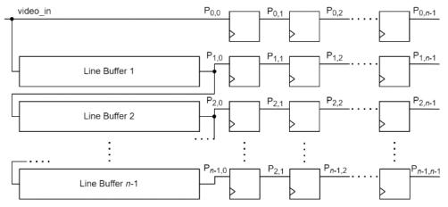
Figure 48. Input pixel matrix for the 2D interpolation kernel
