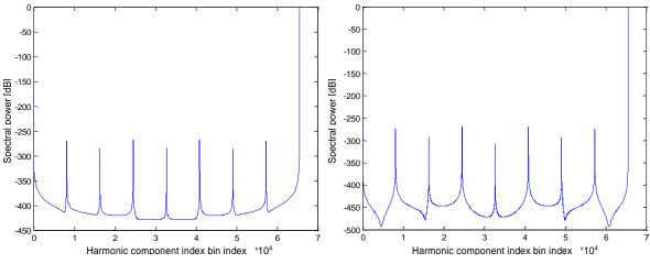
Figure 103. Output spectrum [dB] without (left) and with (right) frequency dithering
