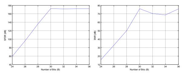
Figure 101. SFDR (left) and SNR (right) as a function of *B*, 18x18 bit multiplier
