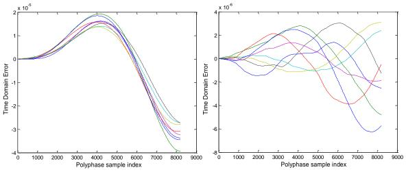
Figure 102. Time Domain error without (left) and with (right) frequency dithering,  $N = 2^{16}$ , p = 8
