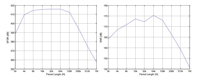
Figure 113. SFDR (left) and SNR (right) of the quadratic interpolator as a function of *N*, *B*=36, *M*=1024
