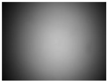
Figure 9: Flat-field image demonstrating strong lens-shading
