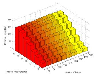
Figure 96. FPR dynamic range as a function of transform size (*N*) and internal precision
