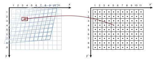
Figure 11: Backward mapping of output pixel positions into the input sampling grid
