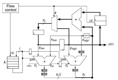
Figure 81. Pipelined bit-serial resonator
