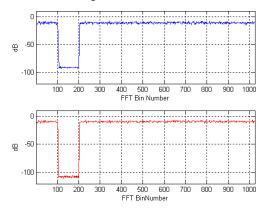
Figure 94. FFT Dynamic range (N=1024, blue: 18-bit fixed-point, red: double precision)
