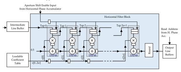
Figure 16: Example of a horizontal scaling FIR filter stage, implemented using DSP48 primitives
