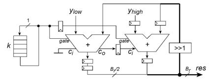
Figure 80. Pipelined bit-serial multiplier
