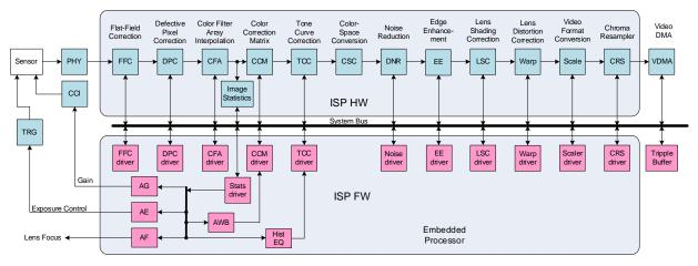
Figure 4: Streaming ISP pipeline HW and FW components
