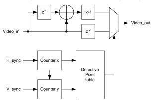
Figure 43. Static solution for Stuck Pixel Correction
