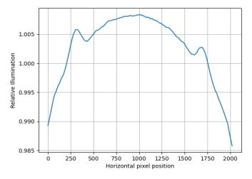
Figure 40. HIP of hybrid lens, 0°C corrected with 60°C
