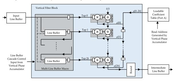
Figure 15: Example of a vertical scaling FIR filter stage, implemented using DSP48 primitives
