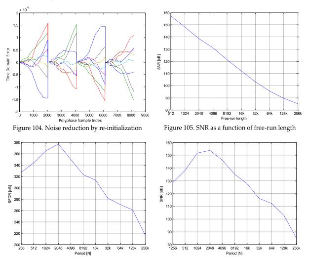
Figure 106. SFDR (left) and SNR (right) as a function of N (35x18 bit multiplier)
