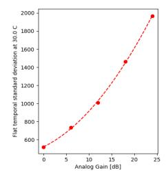
Figure 33. SD of Shot noise as a function of analog gain ( $\alpha$ )
