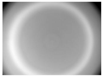
Figure 39. Hybrid lens at 0°C corrected with 60°C image
