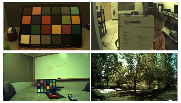
Figure 57: Reference images with four different illuminators top-left: Incandescent, top-right: warm fluorescent, bottom left: cool fluorescent, bottom-right: daylight
