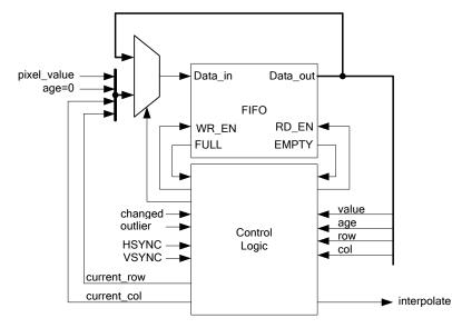
Figure 47. Block Diagram of an FPGA implementation
