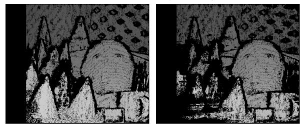
Figure 22. Matching Density with (right) and without (left) FPN
