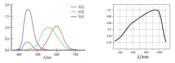
Figure 49. Normalized spectral responses of the CIE Standard Observer, and silicon photodiode
