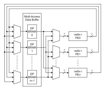
Figure 67. Loop-engine implementation
