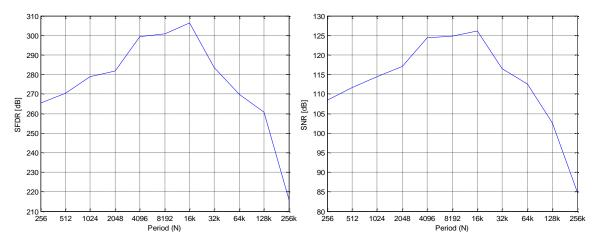
Figure 111. SFDR (left) and SNR (right) as a function of N, 18x18 bit multiplier
