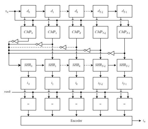
Figure 62: Word-serial filter core architecture
