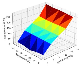
Figure 37. Residual SD of PRNU, single reference correction
