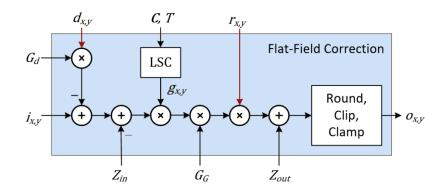
Figure 25. Flat-Field Correction module block diagram
