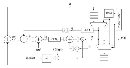
Figure 107. Resonator structure with re-initialization support
