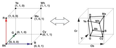
Figure 8: Conceptual conversion between the RGB and YCrCb color-spaces<sup>10</sup>
