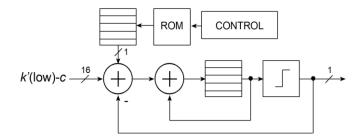
Figure 109. Modified  $\Delta\Sigma$  converter
