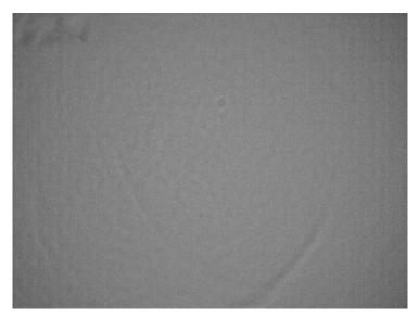
Figure 24. Static integrating sphere image artifacts
