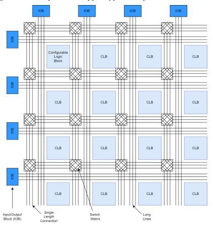
Figure 1: Simple Sea of Gates FPGA architecture.
