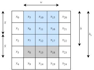
Figure 65: Virtual filter window with padding pixels
