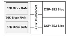
Figure 74: Xilinx Ultrascale BRAM, CLB and DSP48 slice tile
