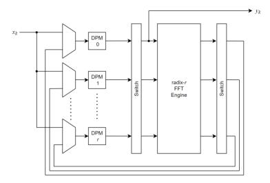
Figure 70. Single buffer Radix-4 FFT loop engine
