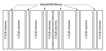
Figure 66. Dedicated resources inserted into the logic fabric
