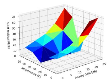
Figure 38. Residual SD of PRNU, multi-reference correction
