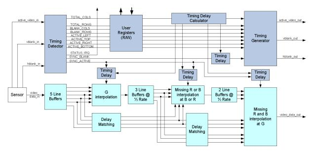
Figure 86. Block diagram of a Color Filter Array Interpolator
