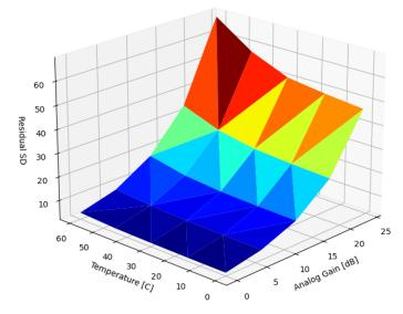
Figure 27. Standard deviation of uncorrected DSNU
