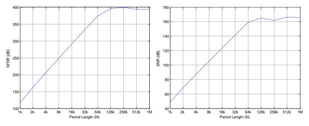
Figure 82. SFDR (left), and SNR (right) for the resonator + quadratic interpolator, as a function of N
