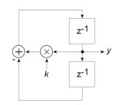
Figure 75. Two-pole resonator
