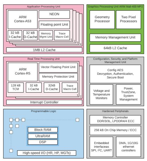
Figure 2: Example block diagram of a modern FPGA device<sup>1</sup>.
