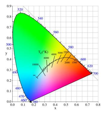
Figure 56: x and y coordinates of illuminants with different temperatures in CIE color-space
