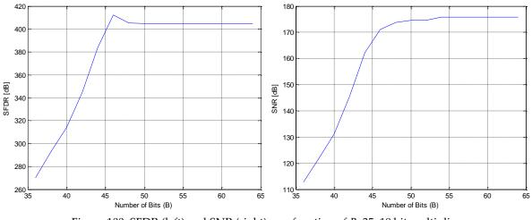
Figure 100. SFDR (left) and SNR (right) as a function of *B*, 35x18 bit multiplier
