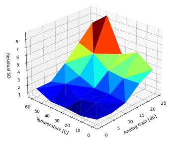
Figure 32. SD of DSNU corrected with interpolation between 5 reference captures
