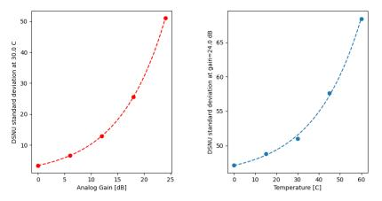
Figure 28. SD of DSNU at 30°C (left), and at 24.0dB gain (right)
