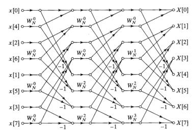
Figure 91. FFT architecture with similar stages
