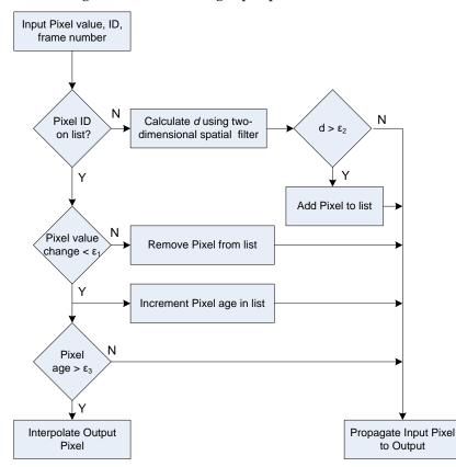
Figure 45. Simplified flow-chart of the proposed algorithm
