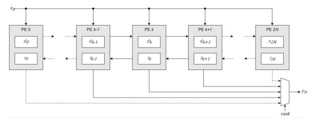
Figure 60: Block Diagram of a 1D rank-ordering architecture
