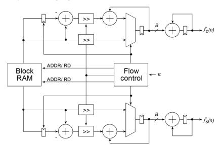
Figure 112. Phase factor source for in-place FFTs based on DII structure
