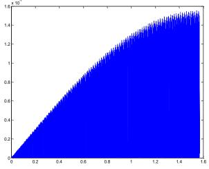
Figure 97. 1407 point linear interpolation, time domain error
