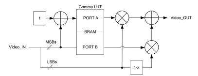
Figure 7: 12 bit gamma correction module with interpolation
