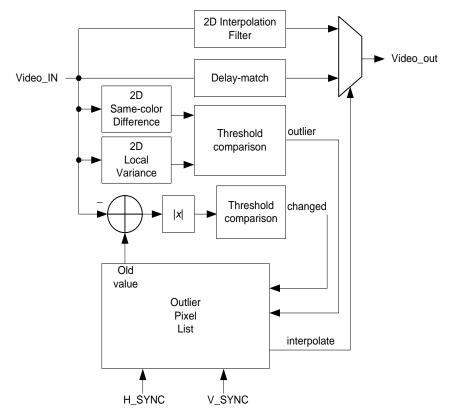
Figure 46. Block Diagram of an FPGA implementation
