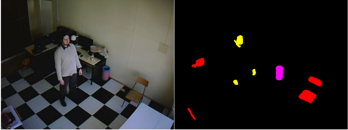
Figure 6.9: A training image (left) and the corresponding mask that marks the different classes (right).
