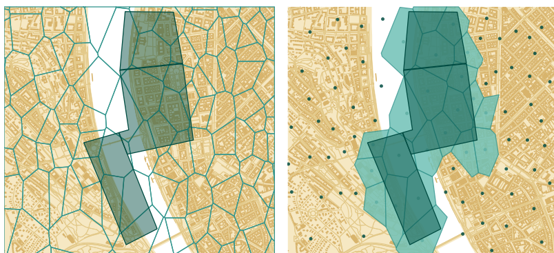
(a) The observation area and the Voronoi polygon representation of the cells.
