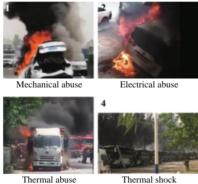
Fig. 21 Actual Li-ion battery related vehicle accidents [58]
