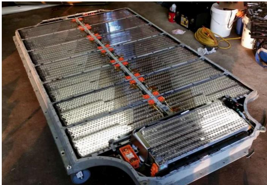
Fig. 2 Tesla Model S standard 100 kWh battery pack [4]
