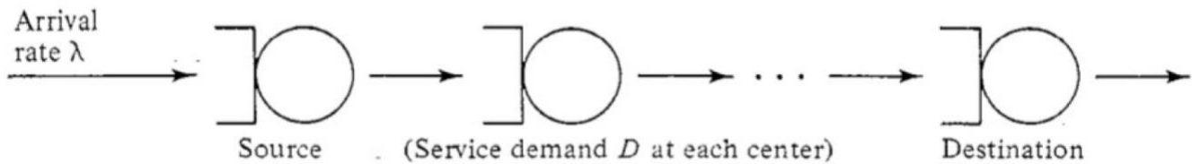
Figure 2.2 Transmission elements [LAZ84]
