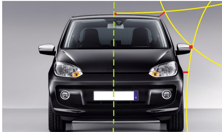
Figure 39: Rolling sphere design for a commercially available car (Edited by author)
