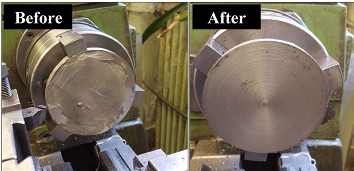
Fig. 4.3. Photo of the sintered 316L composite disc. a) before and b) after the removal of the exterior surface.
