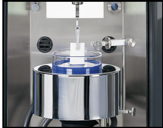
Figure 4.1: Tensiometer (NIMA Ltd, Model DST 9005).
