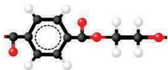
Fig. 1. Chemical structure of PET [4]
