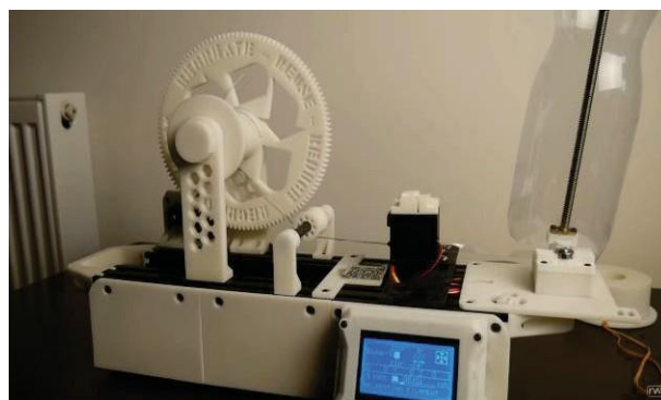
Fig. 6. The filament production process from PET bottle
